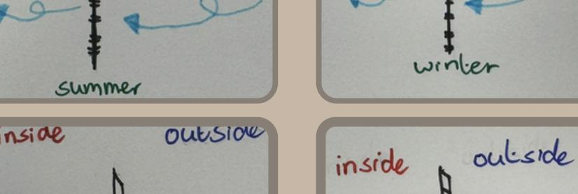
We chose the dynamic louver system because of its seasonal flexibility, natural ventilation, and adjustable daylight. The system combines comfort with cultural aesthetics and operates without additional energy consumption.
