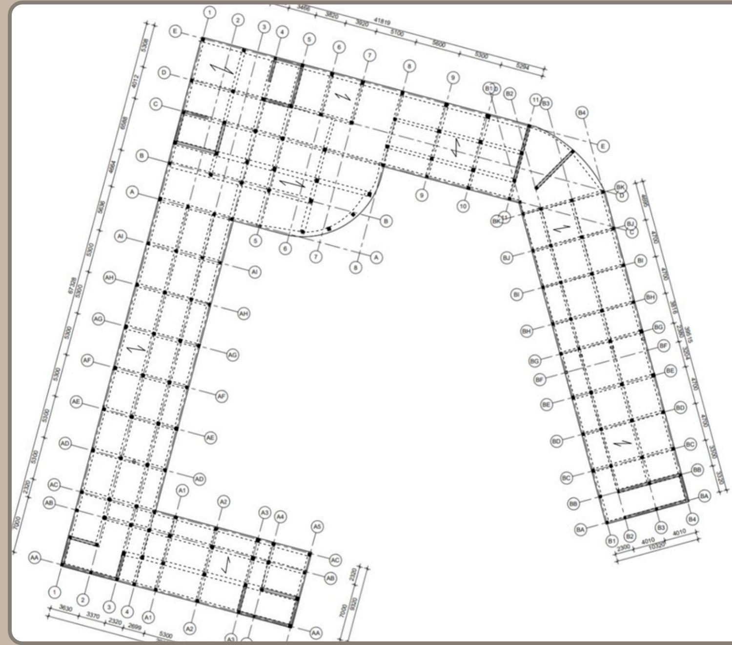
The building design incorporates 320x320 mm columns, with a maximum span of 5.3 meters, for the beams. The structural stability is ensured through the placement of stairwells. Each section of the building is equipped with two stairwells, which serve as key stabilizing elements within the structure.
